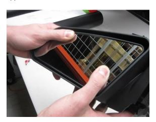
**Step 13:** Install the mirror back on the vehicle using the three nuts removed in Step 6. Once the mirror is mounted, repeat Steps 1-5 in reverse to re-install the speaker and door panel assemblies.
