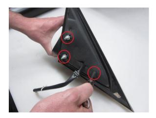
**Step 8:** Remove the mirror glass by using a flat head screwdriver and carefully releasing the tabs securing the glass to the motor.
