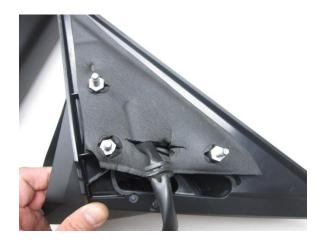
**Step 12:** Install the provided mirror onto the motor as shown. Press firmly around the outer edges until the clips snap into place. Do not press directly in the center of the mirror, this could cause the glass to crack. Be especially careful on the passenger side mirror as the convex glass is slightly raised in the center, making it more prone to flex when pressure is applied.
