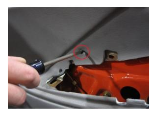
**Step 4:** You can now remove the door panel by firmly pulling up and away from the door. Be sure to maneuver the panel around the interior door handle as shown.
