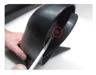
**Step 9:** Remove the motor from the mirror housing using a T10 Torx driver. It may help to unplug the harness from the motor before removing the harness from the mirror housing.
