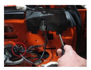
**Step 6:** Using an 11mm socket, remove the three nuts securing the mirror to the door and remove it from the vehicle.
