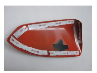
**Step 16:** Peel the backing from the tape and place the cover over the mirror starting with the inside part of the cover. Once the cover is properly positioned, press down firmly to fully seat the adhesive tape.
