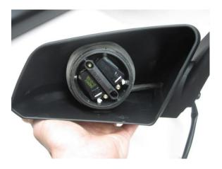
**Step 11:** Install the foam insulator and factory mounting studs onto the new mirror as shown.
