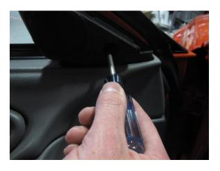
**Step 3:** Remove the retaining clip at the front of the door panel along with the Phillips head screw shown in the photo below.
