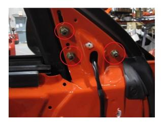
**Step 7:** You will re-use some of the parts from your factory mirror in the installation of your new mirror; the mounting studs, the foam insulator, the motor and wiring harness, and the motor retaining screws. Remove the mounting studs using an 11mm socket. Then remove the foam insulator.
