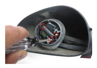
**Step 10:** Plug the harness back into the motor and mount it in your new mirror using the factory screws. Tighten until just snug, do not over tighten the mounting screws.
