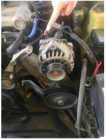
7. Now remove the bottom 15mm bolt loosened in step 5 and remove old alternator.
