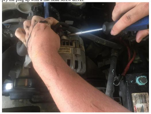
4. Use the 13mm socket to remove top bolt holding the alternator in place.
