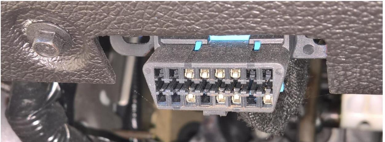
6. Connect the ProCal tool to the diagnostics port while pressing Enter. The tool will update itself with the software from the memory card. Do not continue to the next step until the red error light goes out and the menu appears reading "Programming / Diagnostics / Vehicle Setup."
