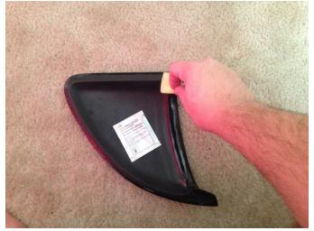
**STEP 2:** Apply the supplied 3M tape to the back of the scoop, press it down and allow it to set for 5 minutes.
