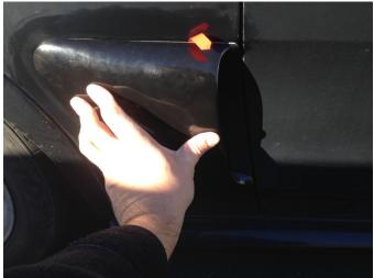
**STEP 6:** Peel the backing off, while holding the scoop still, until the entire length of red backing is removed, then press the scoop tight against the car and allow it to set.
