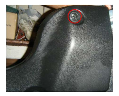
3. Using the 11mm socket, remove the (3) nuts that hold the tail light to the body. You can use a wrench if you don't have a deep socket and ratchet, but it will be a just a little more difficult.
