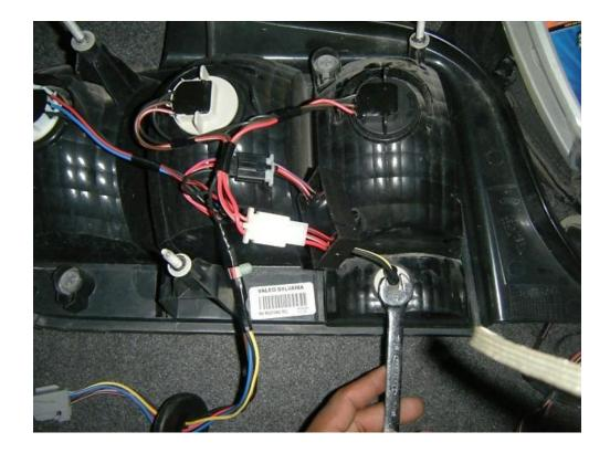
7. Once you reconnect the plugs in the taillight, make sure the rubber gasket has been pushed into the hole untilit is flush with the body. This is important to provide a water tight seal. Connect the wiring harness.
