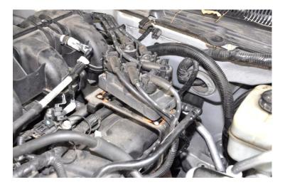
You need to swing the evac hose, pictured above against the HV wires, out of the way. I found it easiest to disconnect the hose at the OTHER end and just swing it up out of the way.
