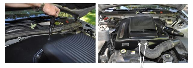
The Throttle Body bolts are under here
