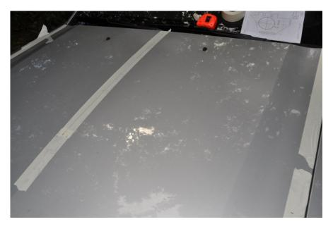
Here the instructions say to cover the entire scoop area with tape and then tape the template to the hood. In my case, I elected to NOT use the original template, but instead used a copy machine to copy the original template onto 4 separate sheets of paper. I then placed each of the sheets on the hood in the position indicated.
