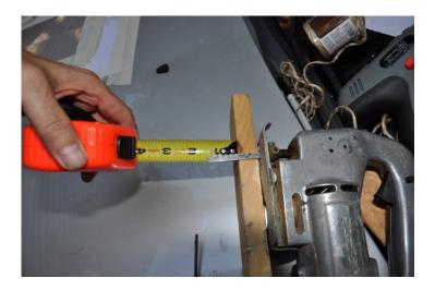
Drill a ¼" or larger hole inside the cutout area to start the blade and then carefully follow the template marking for 1 side only. Once you cut one edge, use tape over the cut to make sure the metal cannot 'flop around' as you cut. Carefully cut the
