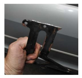
One the bracket is cut, mount the supplied piece to the bracket with the button head screws and flange nuts. Put the bracket together loosely and attach it to the
