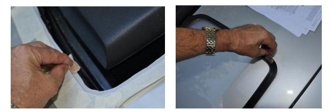
Invert the trim ring and sand the underside that will be out of sight. It is not necessary to sand the 'lip'. You want to sand the flat area under the trim ring, specifically toward the lip on the edge. Shortly you will be placing a tape in the flat groove.
