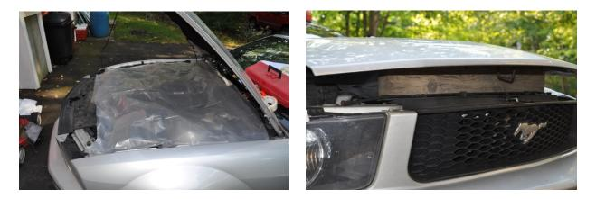
The original instructions recommend removing the thermal blanket from the underside of the hood, but I didn't have access to a fork tool and elected to just cut from the top. I used a hand electric sabre saw with a fine pitch 24tpi (tooth per inch) metal blade. I also used a piece of wood furring strip to offset the sabre saw so at to limit the penetration of the blade below the hood.
