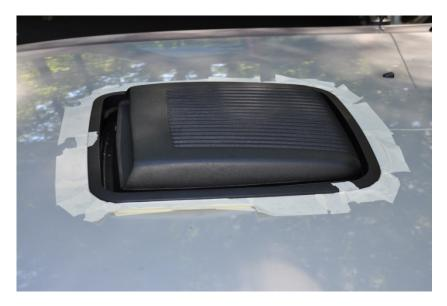
Once the trim ring is outlined, carefully remove the tape holding the trim ring in position and finish the outline in the areas previously covered by the hold-down tape. Once you are satisfied, gently lift out the ring and make sure your 'tape outline' on the hood is complete with no gaps.
