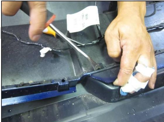
15. Install RTR Diffuser/Splitter to rear fascia, reversing the procedure outlined above. Begin by installing all locking tabs of diffuser/splitter into rear fascia, pressing firmly in place with thumbs. Reinstall push pins, screws, and push pin wire harness retainers. Once complete, turn fascia over to inspect and ensure all tabs have been properly seated. Note locating pins on fascia (circled below).
