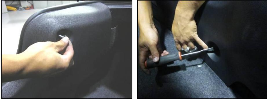
2. There are two hidden fasteners and locating pins located beneath the top of the trim panel. Using hands, carefully lift upward and forward on the panel, releasing the fasteners. Use caution as trunk courtesy light is attached to panel and wire harness has limited length. Lean panel forward in trunk; it does not need to be completely removed; only need to gain access to taillight mounting bolts.
