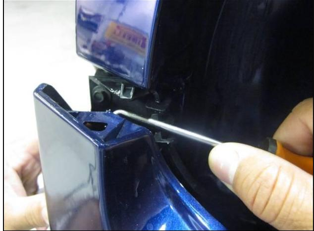
12. Four large push-pin type retainers remain at the center of the fascia (circled). With the use of a friendly assistant (one person per side of fascia), secure fascia so that left/right ends will not hit quarter panels during removal process. With free hands, pull fascia swiftly rearward to dislodge 4 remaining fasteners. Guide previously disconnected harness through hole as you remove fascia from car. Place fascia on soft surface.
