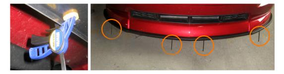
4. Align the splitter to the desired position making sure that it is centered and flush to the back if desired. There should be about 1'' of the splitter on each side of the spoiler.
