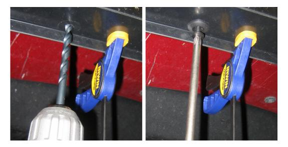
6. Continue drilling and installing the retainers through the holes in the splitter, moving outward alternating sides as you go. Move your clamps so that they are holding the splitter tight to the spoiler and do not focus on just one side of the splitter.
