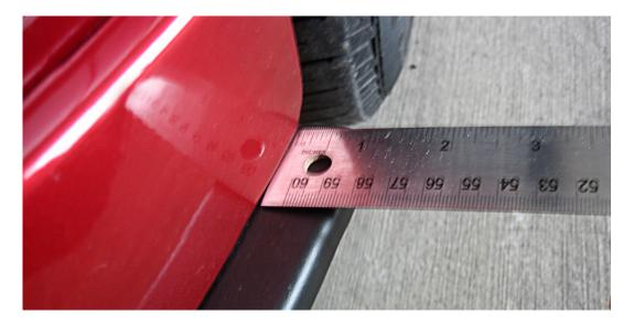
5. Once in position drill through the chin spoiler at the center hole using a 1/4 bit and install the plastic screw in retainer that is supplied with your splitter
