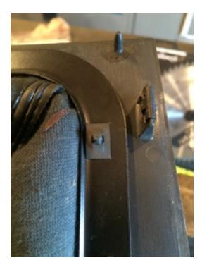
Step 5 continued: Once removed keep the 4 retaining clips separate.
