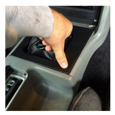
Step 5: Re-install the shift knob by twisting clockwise.
