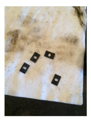
Step 6: On the old bezel there are 4 clips that will need to be transferred to the new bezel in order for it to snap into place on the center console. With your hands pull the Clips off the bezel. If it is too hard for your hands, use the flat head screwdriver to aid you.
