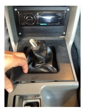
Step 3: Pull up on the remaining corners of the shifter bezel until it is free.
