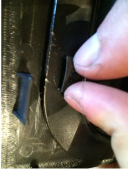
Step 3: With the shifter boot attached to the bezel, place over the shifter and slide the shifter boot down onto the shifter.
