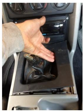
Step 4: slide the shift boot over the shifter, the shifter bezel and boot are connected together.
