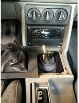
Step 5: Next you will need to remove the Shifter boot from the bezel. The boot is held to the bezel by 4 Clips. Using a flat head screw driver pry the clips off the bezel.
