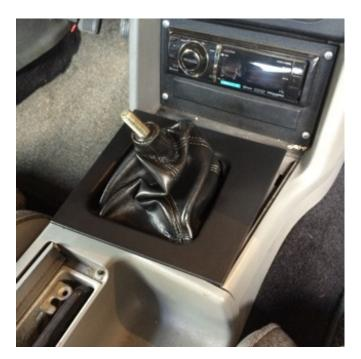
Step 4: By pressing down snap the new bezel into the center console one corner at a time.
