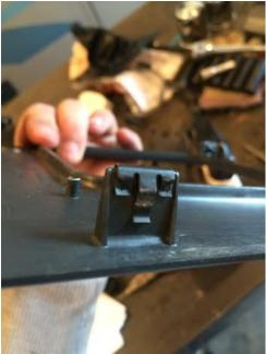
Step 2: Next you will need to install the shifter boot to the new bezel, Line the boot holes up with the corresponding tabs on the bezel and press the retaining clips over the tabs.
