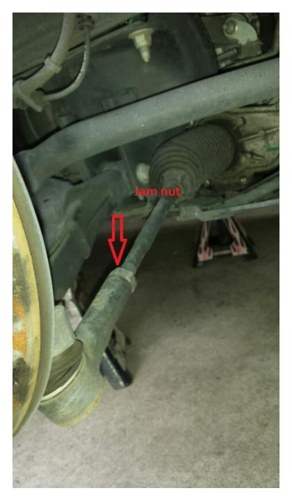
4. Unscrew the heavy nut holding the outer tie rod to the hub assembly, and unscrew the outer tie rod from the inner tie rod as shown.
