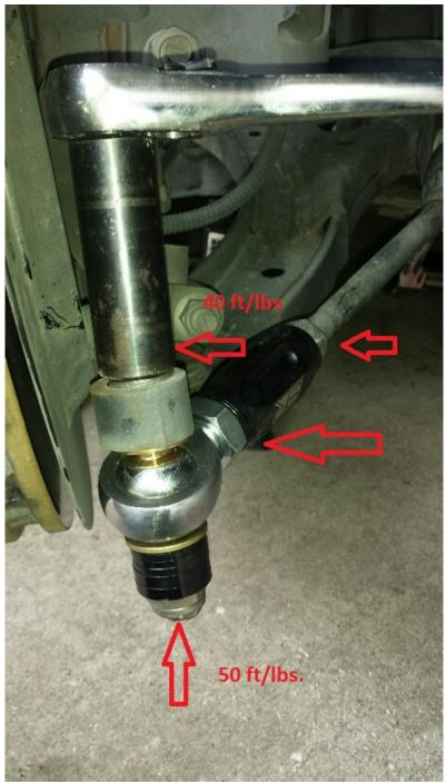
8. Install wheels and have alignment checked. Check all torque on nuts after installation and after first few hundred miles to insure nothing has backed off.
