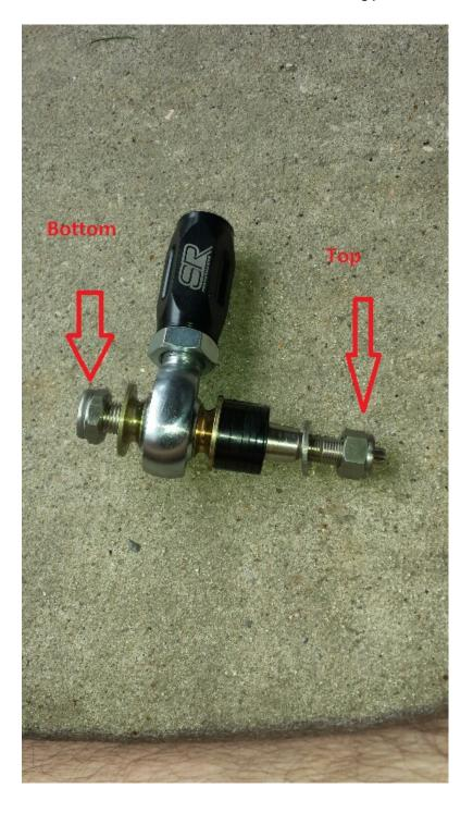
7. Using the smaller and larger adjustable wrenches, tighten the 2 jam nuts towards each other. Install the bolt assembly according to step #6 and tighten the two nuts (upper and lower) to the stated torque ratings. Repeat these steps on the opposite sides to complete the installation.
