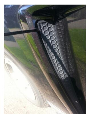
2) Open up the packaging containing your new inserts. Peel back the red 3M plastic backing.
