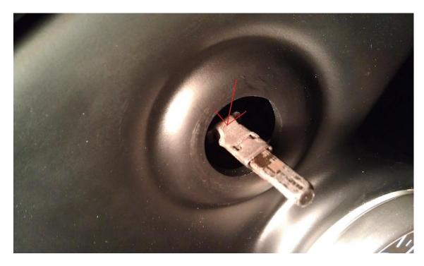
3. Take the t20 torx and remove the (2) holding screws up at the topside of the bezel.
