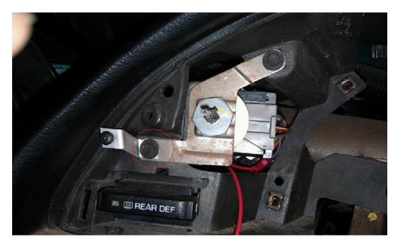
6. The long bracket goes on the lower right side of the instrument cluster. This one mounts in the place of the lower right screw that holds the instrument panel in place. Take your t20 torx and remove that screw then use it to mount the long bracket. It should look like this when installed.
