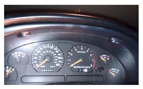
11. Now take the (2) mini screws supplied with the new autometer bezel screw them into the brackets we installed with your t10 torx screwdrivers. If the holes in the bezel and brackets don't line up, you can bend the brackets until the do. Screw in the left and right ones to look like this.
