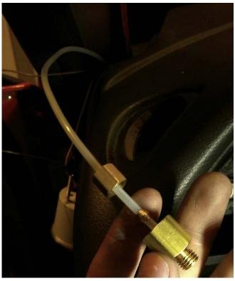
**9.** Tighten the brass fittings using a  $\frac{1}{2}$ " and  $\frac{3}{8}$  wrench. Make sure the fittings are snug, to avoid vacuum leaks.
