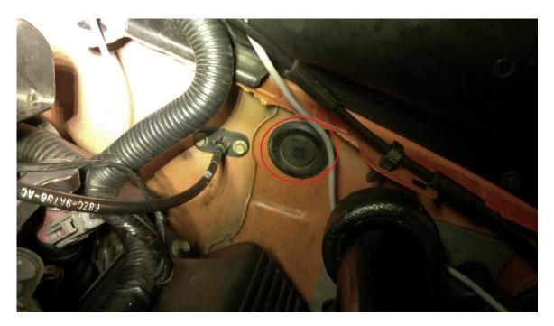
3. NOTE: on some Mustangs, the clutch cable may not allow room for the vacuum tube to pass through the grommet. Alternatively, you can use the grommet for the hood cable, shown below.
