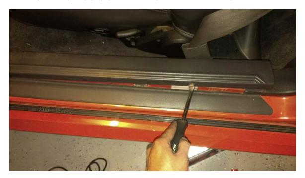
9. Next, remove the driver's side kick panel. Using the trim tool, or a screw driver, first remove the plastic push pin holding the kick panel in place.
