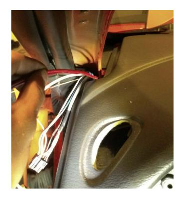
NOTE: if you are installing more than one gauge in the A pillar location, you may find it necessary to use a Dremel tool, or file, to slightly elongate the hole between the dash and the body of the car. This will be totally invisible with the A pillar installed.
