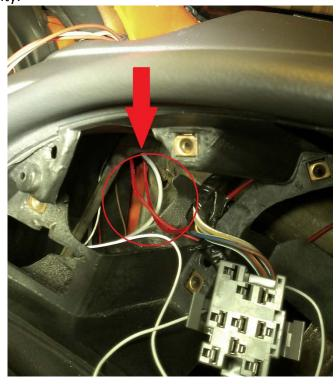
**14.** Take your  $^{7}/_{64}$ <sup>th</sup>, or other small drill bit and make a small pilot hole in the dash frame in the location shown.
