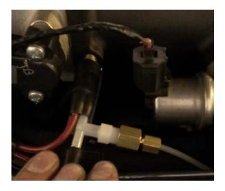
26. Zip tie the vacuum line out of the way, and coil any excess under the dash.
