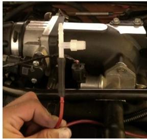
25. Install the 'T' fitting into the black rubber fitting, and install the brass fittings onto the white vacuum hose going to the boost gauge, as shown.
