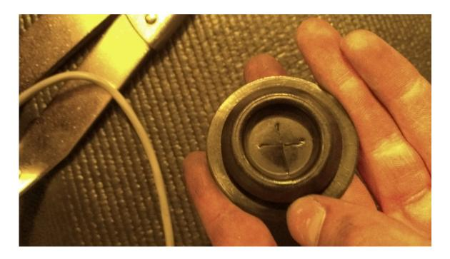
**5.** Route the vacuum tube for the boost gauge through the grommet, into the firewall, as shown.
