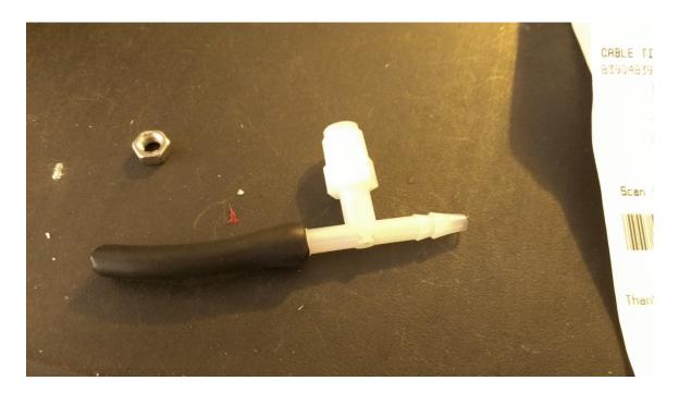
24. Remove one of the red vacuum tubes from the black rubbing fitting, and replace it with the 'T' fitting, as shown.
