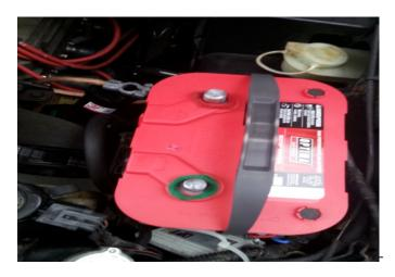
**12.** Put your positive (+) battery terminal back on, and tighten it with your 13mm wrench. Then put your negative (-) terminal on (13mm wrench too).
