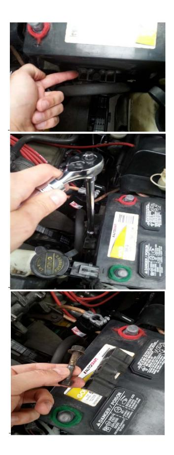
**6.** Once you pull the battery out, you will have full access to the battery tray. To see how your new Optima battery will fit, test it with that red top that you pulled off earlier. I did not need to cut or modify anything at all. But apparently, the owner before me did cut the tray. This happens to be the spot that every other model has to cut in order to get the battery to fit.
