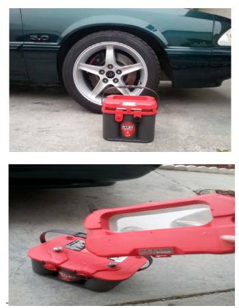
**3.** Before you begin, NOW is a good time to learn and memorize where the positive (+) and negative (-) outputs are on the battery. With regards to the Foxbody (this car), the positive output is the wire that is toward the rear of the car (the clear wire with the red circle on the terminal), and the negative output is black wire (with the green circle) that is toward the front. Notice the "+" and "-" symbols on the battery and which wire they are connected to.
