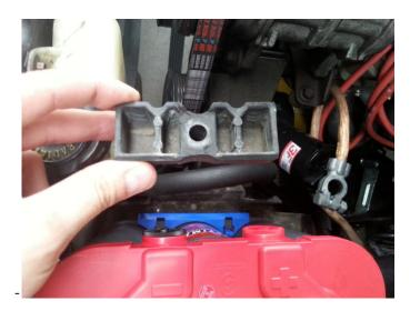
**10.** Grab your socket wrench with the 13mm socket on it, and put the nut and bolt back on. Be SURE that the battery does not wiggle or cannot come loose.
