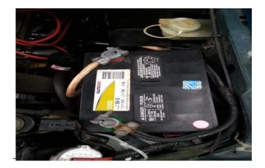
**4**. To remove the old battery with your 13mm wrench. Start with the NEGATIVE (-) terminal. Remember to put the wire in an out of the way position and a safe location. Take the positive (+) terminal off the same way.
