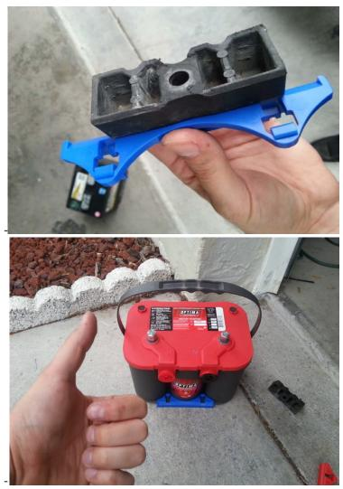
**9.** Place your new Optima battery in the car and make sure it fits. You do not want it to be loose. Be sure that the positive side (+) and the negative side (-) are facing the same way as before. Put the plastic piece in the holds the battery down in place. Be sure that everything is tight and fits properly.
