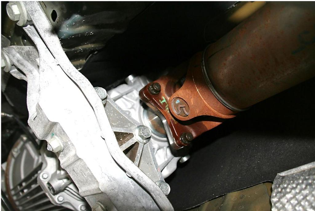
3. Put the car in gear and put the emergency brake on. Go under the car and remove the (4) visible bolts with your breaker bar and 12mm socket. **Note:** some breaker bar heads will not clear the small space and a universal joint or an extension is necessary to fully remove the bolts.
