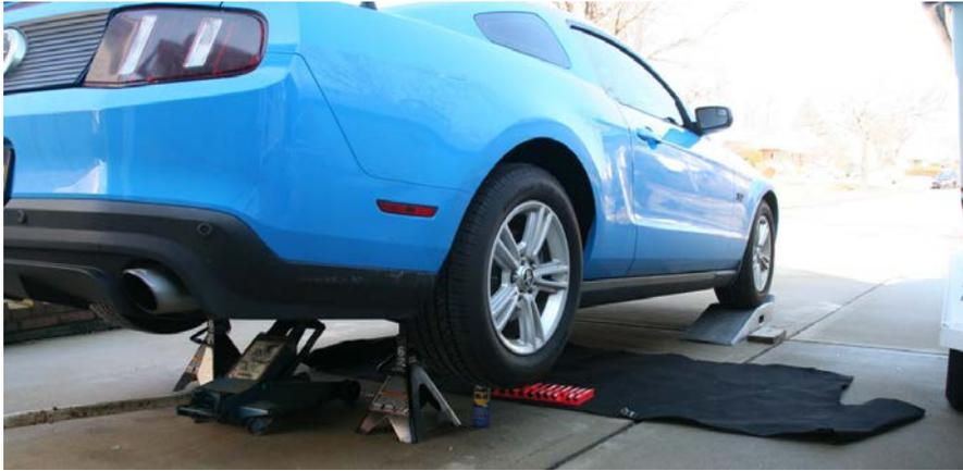
2. Put the car in neutral and leave the emergency brake off. Go under the car and spray the (8) bolts that hold the driveshaft in place with WD-40 or PB Blaster. There are (4) bolts on the transmission side and (4) bolts on the rear end side; only (2) of each will be visible and then you must spin your driveshaft with your hand to get to the other two.
