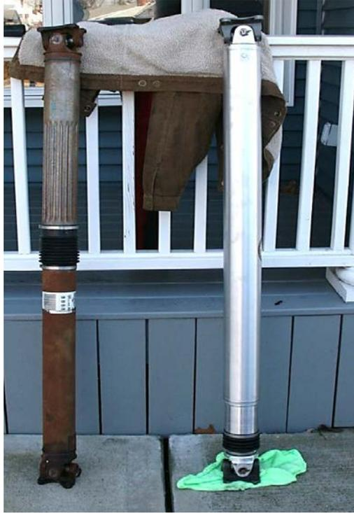
8. Take (4) of the bolts and put Loctite on them. Install them in their place on the transmission and rear-end side of the driveshaft. Torque them down to 75 lbs/ft with your torque wrench.
