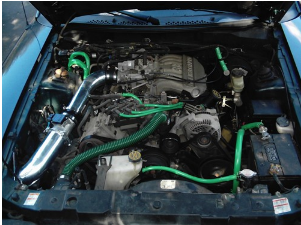
After: New Cold Air Intake
