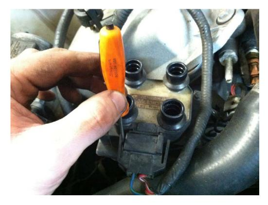
**3:** Remove the 4 bolts from the coils using a 7mm socket.
