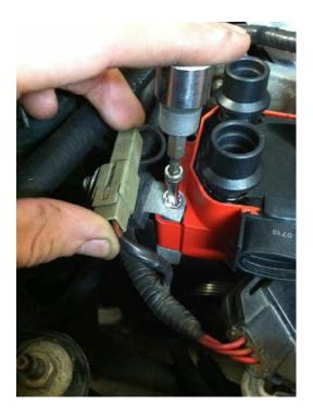
**6:** Reinstall the electrical connectors to the MSD ignition coils.
