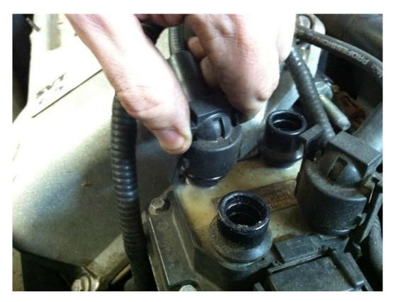
**2:** Remove the electrical connector from the old coils. A small screwdriver will make this easier. Just be careful not to break the clips.
