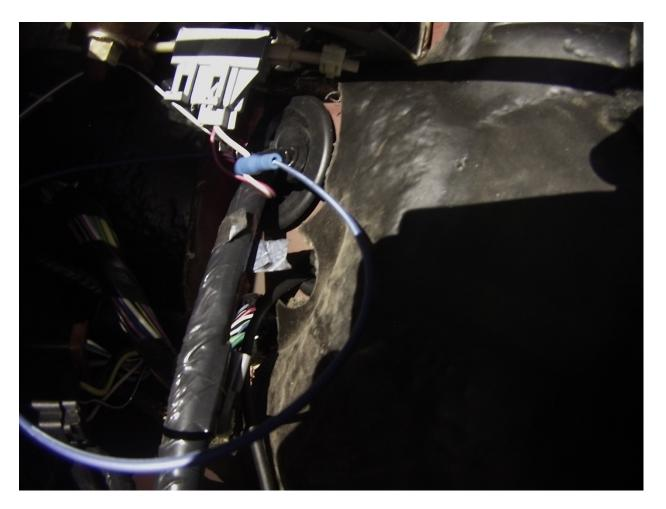
11. After this step the installation is complete! Reassemble the covers on top of the coil and you're done. To set the 2step you must use the dials on the side of the box, to the left is the 1000's, and to the right is the 100's. The blue-white wire is not used!
