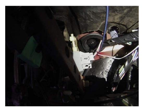
10. Choose any of the two wires off the switch and use the easy crimp on the wire tapping the BLUE wire to the module
