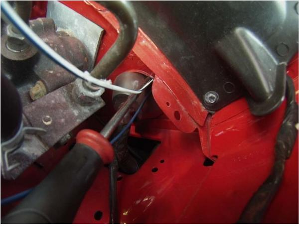
9. Locate the clutch switch. The clutch switch is on the top of the pedal. You will see two wires going into the top of the switch
