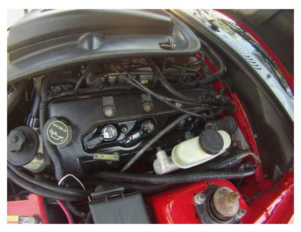
4. Disconnect all of the plugs from the coils. Plug the wire you disconnected off of the coil in the harness. Then plug the wire on the harness into the coil. The wires are self explanatory the longest one goes to the front of the motor, and the shortest one goes to the back of the motor.
