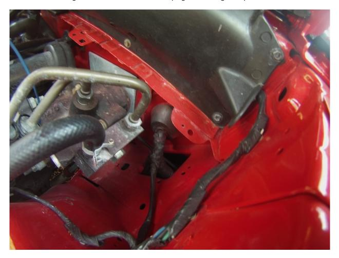
8. Place a flat head screwdriver in the grommet to make room to slip the wires threw the firewall
