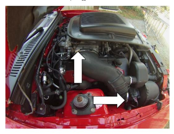
3. Remove the two 10MM bolts and the coil covers will come right off!
