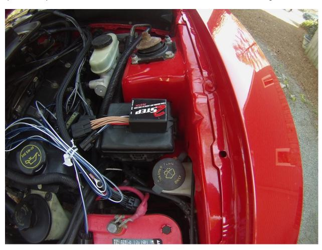
6. Grounding the module - Place the black wire to the negative side of the battery.
