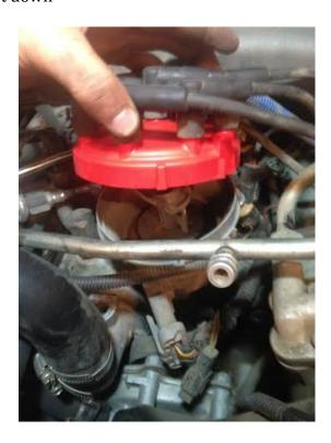
Step 6: Push the levers back over the cap so it's secured to the distributor
