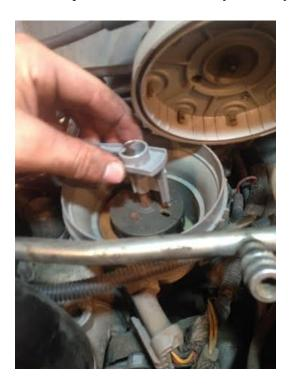
Step 2: Next take the new MSD cap and make sure it is oriented correctly. There is a square notch on the edge of the MSD cap, make sure this notch is in the same position as the old cap.
