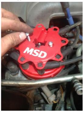
Step 5: Snap the Center wire into the Cap.
