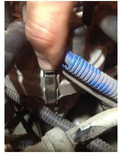
Step 2: With the two levers released pull the cap off the distributor exposing the rotor  ${\bf r}$
