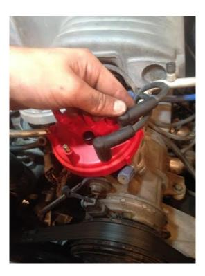
Step 5: After all wires have been transferred to the new cap, line the cap up with the distributor and set it down
