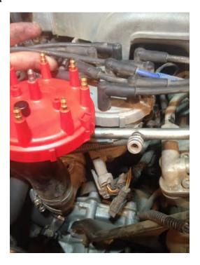
Step 3: With the cap oriented correctly take the plug wire to the left of the notch and transfer it over to the MSD cap from the old cap.
