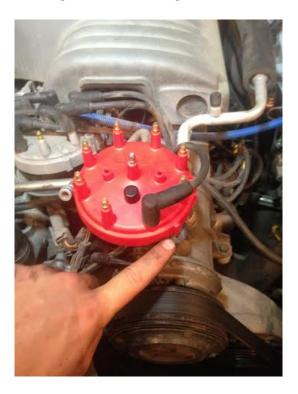
Step 4: With the first wire transferred over, start by going counterclockwise transferring all of the other wires to the new MSD cap.
