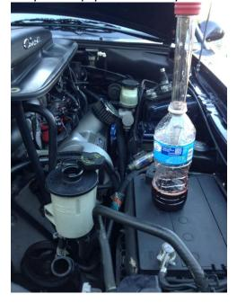
2. Once most of the fluid is out of the reservoir, take your pliers and, one at a time, pinch the clamps holding the two hoses onto the reservoir. Slide the clamps far enough down the hose so they are out of your way.
