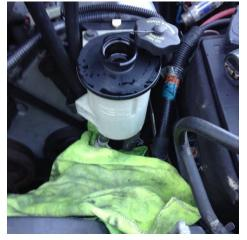
hoses that attach to the bottom of the reservoir. Give them a good pull and they should slide right off. Have your rags ready as a little bit of excess fluid will pour out of the reservoir and lines.
