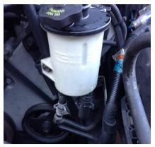
3. Next, locate the three 10mm bolts mounting the reservoir to the engine. 2 of the bolts are directly on top, while the third is on the left side of the tank.
