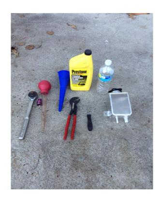
1. Open your power steering reservoir cap. Using your turkey baster suck as much fluid out of the reservoir as you can. Squirt the excess fluid into your empty bottle. Safely discard old fluid.
