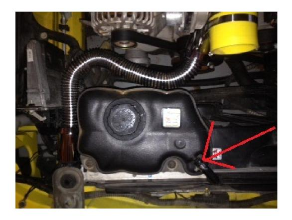
4. Disconnect bottom line from coolant tank. This can be accomplished using the Slip-joint pliers.
