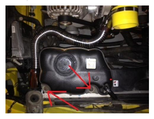
NOTE Have a small container to catch any fluid from coolant tank lines.
