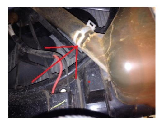
5. Remove stock coolant tank.
