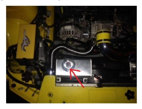
11. Start the engine. Make sure the new Tank and lines are not leaking.
