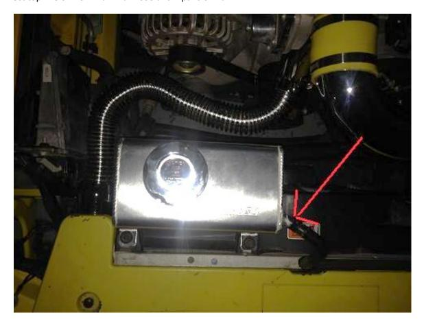
8. Install two bolts on top of new Aluminum Coolant Expansion Tank. Tighten using 8MM wrench/socket.
