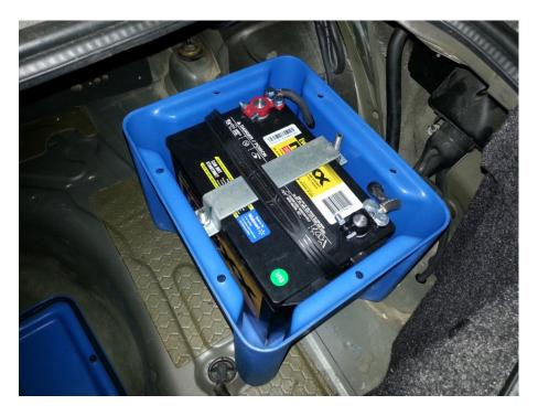
15) Install the lid by putting the Swell Latches through the holes in the box, and push down the tabs to seal the box.
