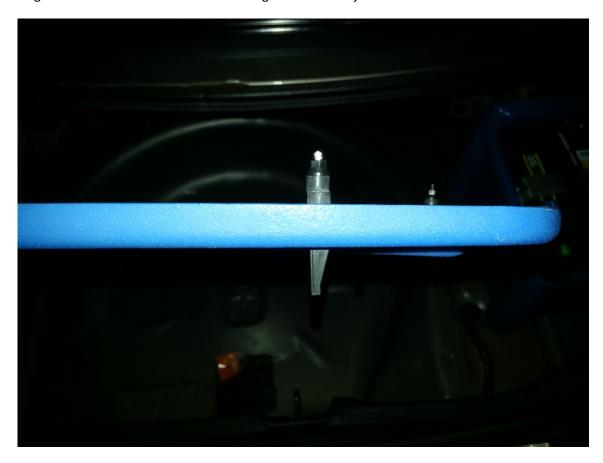
12) Install the vent tube through the grommet in the box and through the trunk floor.
