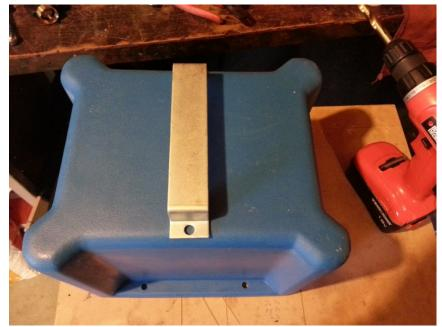
2) Use the hold down bracket again to mark the trunk floor where the bolts will go through the floor. Make sure there isn't anything under the proposed holes that you don't want nicked, cut, or drilled through. Drill the holes.
