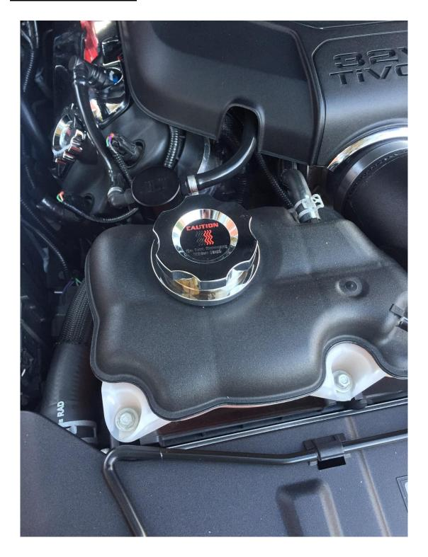
1. Remove the two coolant lines connected to the factory coolant tank using your pliers.
