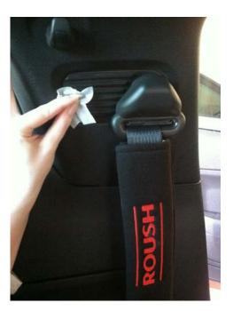
(2) Remove the 3M tape and install. (Note: Be prepared to supplement your adhesion with silicon if needed).
