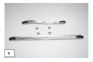
14. Remove the Charge Motion Control Plates, by unscrewing the four (4) Torx screws that attach them to the intake ports (two per side). **Figure 10**
