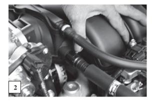
3. Remove all wiring harnesses connected to the intake manifold by pressing the release and pulling the wire from the connection. There are two connectors on the throttlebody, one on the right side for the fuel injection harnesses and one connection behind the intake manifold, next to the fire wall for the actuator motor.
