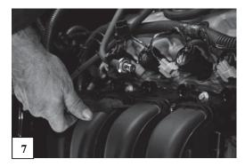
12. Once the bolts are removed, carefully lift the intake manifold from the engine and place on a workbench away from the engine. It is a good practice to cover the intake ports with shop towels until you are ready to reinstall the intake. This will help prevent debris from falling into the engine.
