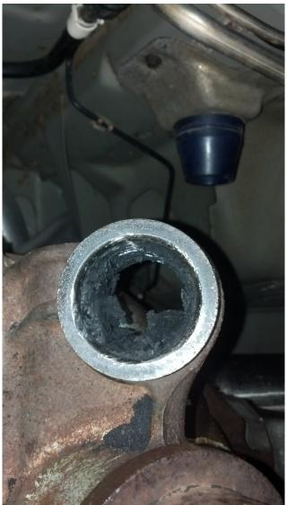
8. Once I got to this point, I found that using a 2" wire wheel worked much quicker and cleaner. I had to slightly modify the new 2" wire wheel using some large pliers to reduce the length of the wires by clamping them down (this is necessary as the bushing's housing is slightly smaller than 2" in diameter). I also sprayed a little WD-40 as I drilled to make this job easier.
