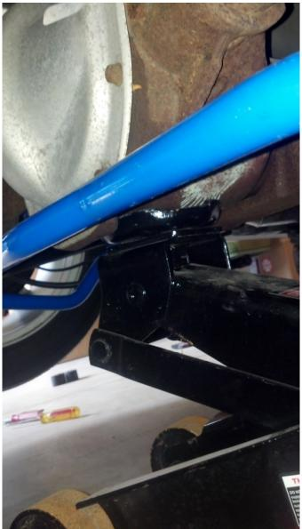
3. Work on one side at the time. Remove the nut from the bolt that connects the upper control arm to the rear axle. Wiggle the bolt out, using the jack to manipulate the height and angle of the axle so the bolt slides out easier.
