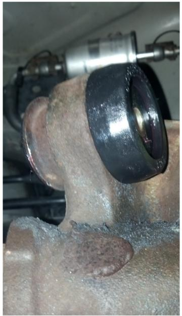
12. Now grease the red bushings on the upper control arm, as well as the contact area in the upper control arm torque box. Bolt the upper control arm up first to the chassis side, then on the axle end.
