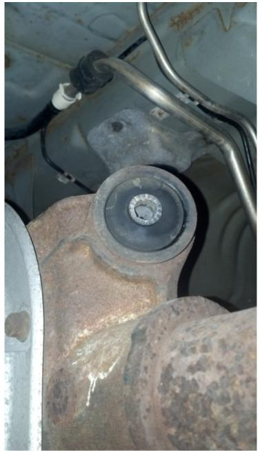
5. Using your preferred method, measure the distance between the bolt holes on the factory upper control arm. This 2002 GT's UCA was right at 9.25". Note: when using a yard stick as pictured, put the 1" mark at the front of the chassis end's hole, and measure to the front of the axle end's hole. Remember to subtract 1" from the measurement.
