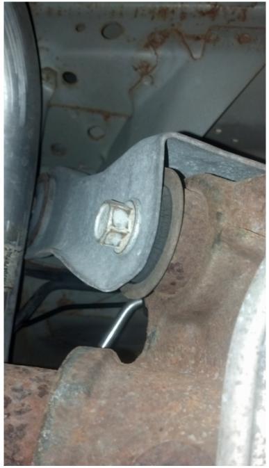
4. Pivot the upper control arm up from the axle, and remove the nut and bolt attaching the upper control arm to the chassis. Remove the control arm from the car.
