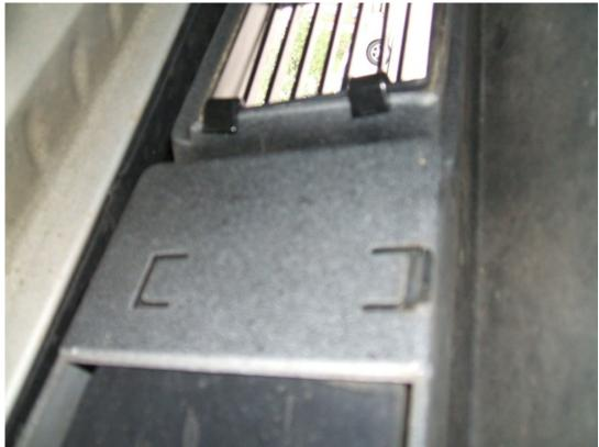
14. Once you have all the "J" hooks securely attached to the factory grille tighten down the screws by going through the Billet grille as shown. **Note: On my lower grille I did have to bend it slightly to get it to fit right**
