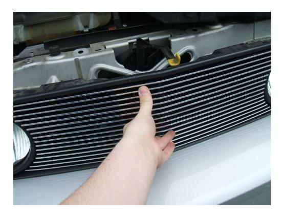
6. Use the supplied 4 bolts, the 4 flat tabs, and the 4 locking nuts to secure the grille in place. Make sure it is still lined up how you want it and then tighten all the bolts.
