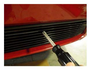
**Step 5:**Once all of the hooks are secured around the factory bumper, use a Phillips head screwdriver and a deep socket to hold the nut and tighten the screw.
