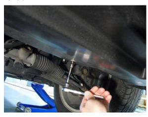
**Step 2:**Use the (2) U-brackets on the outer mounting locations. Use the (2) J-brackets on the inner mounting locations.
