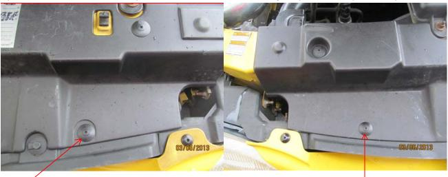
2. If you place a flat screwdriver under the lip and apply pressure upward it will allow the plastic Phillips screw to come out easier.
