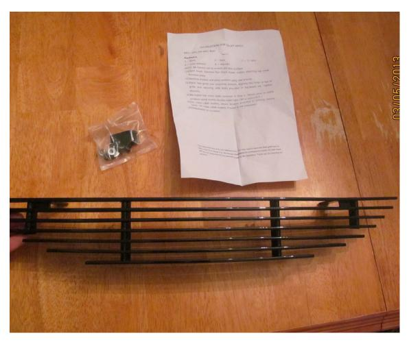
4. You will place the new grill into place to ensure the holes line up. Start by installing the bolt and nut on one side, leave it lose so you can move the grill around to align the bolt hole on the other side. I used a 3/8 drill to enlarge one side. The bolts holes did not line up perfectly. I used the drill to ream out the plastic hole a little. See photo below where holes to mount grill are (I only had to ream one out a little).
