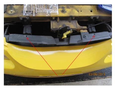
5. You will need two 10mm wrenches to tighten down the grill bolts. Place one wrench under the grill assembly and one to tighten down the bolt head (see photo below).
