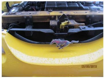
3. It is now time to remove the pony emblem, you will need a star wrench to remove this. You can also drill out the two bolts since this bracket will not be used with the new grill.
