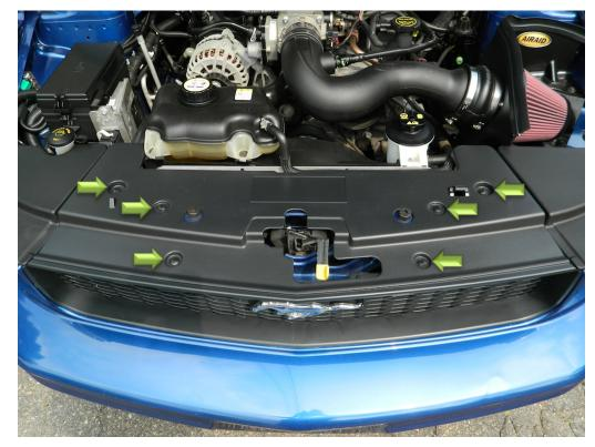
**1.** Open hood and remove six plastic retaining push pins from radiator cover.
