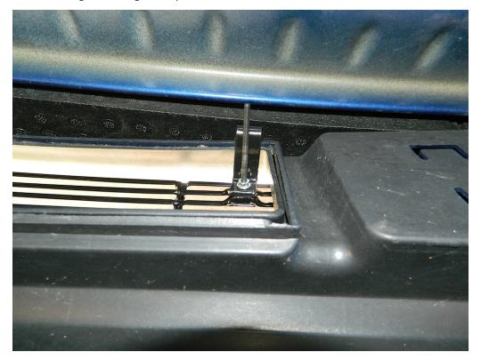
**4.** Attach C-Hooks to both left and right sides loosely, ensure grille is aligned center and fasten in place using a Philips screw driver.
