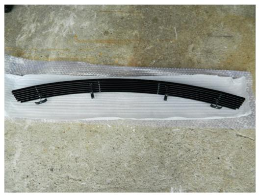
Place Modern Billet Grille overlay over existing lower honeycomb grille. Align middle J-Hooks and tighten using a Philips screw driver.
