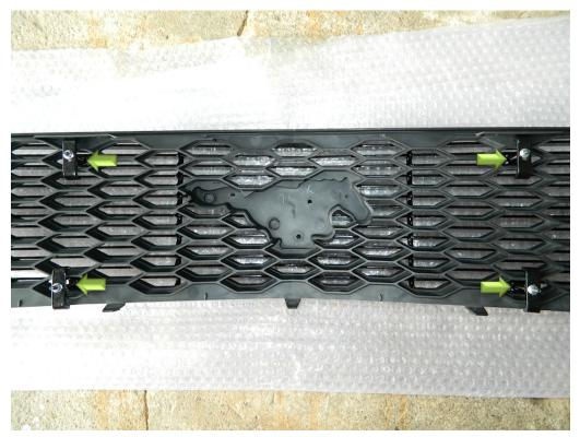
**7.** Reinstall grille back on to vehicle by aligning tabs with bumper cover and press firmly in to place. Reinstall plastic radiator cover and six plastic retaining push pins.
