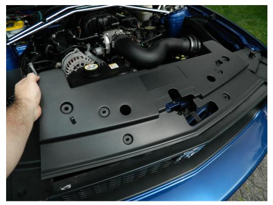
**3.** Remove front grille from vehicle by releasing retaining tab's using a long slotted screwdriver.
