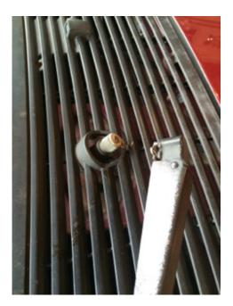
Step 4: With the screwdriver unscrew the 6 screws that hold the cowl to the car.
