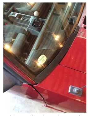
With both Lower trim moldings in place the cowl can now be re installed
