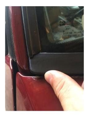
Step 2: There are two tabs on new lower trim that need to be lined up with the two brackets on the car.
