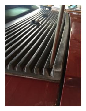
After removing the 6 screws lift the cowl up, you will see a hose going to the sprayer.
