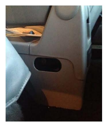
Step 1: Take a flat head screwdriver or a knife to pry one side of the plug out of the console.
