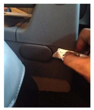
Step 2: Pull the plug completely out of the center console.
