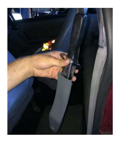
Step 2: After the seat belt is in the new sleeve line up the hole on the end of the seat belt with the hole in the sleeve, insert the bolt and thread it back into the floor using the torx bit to tighten.
