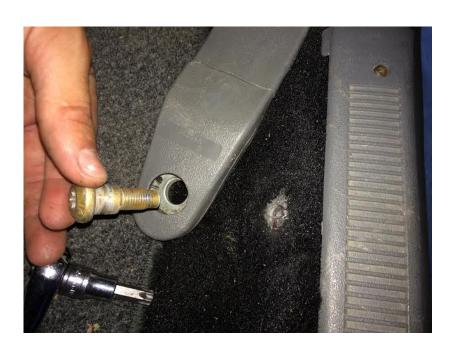
Step 3: Pull the seat belt out of the sleeve.
