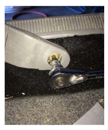
Step 2: Once removed take the bolt out of the seat belt sleeve allowing the seat belt to slide out of the sleeve.
