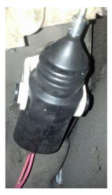
15. Using a rivet gun put a new rivet to hold the actuator motor in.
