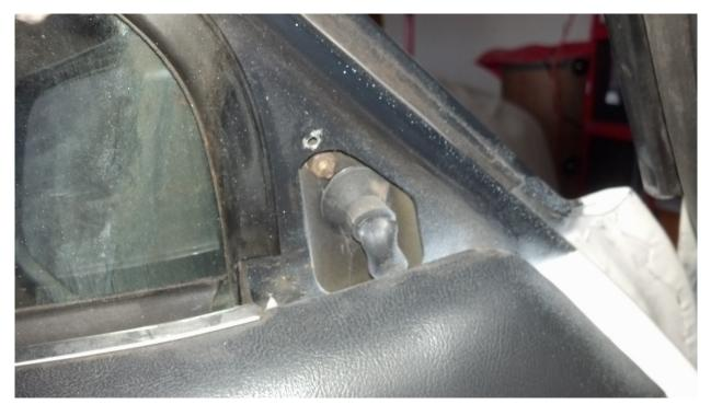
3. Remove the plastic piece from around the door handle with the phillips screw driver.
