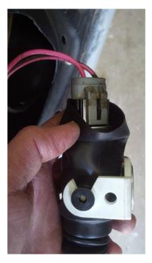
14. Put the actuator in and slide the Z or S style hook in again you will need to slide it up and around a little bit to get it to go into place.
