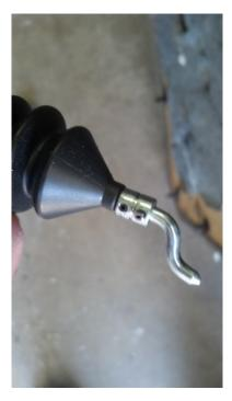
13. Attach the wire clip to the new actuator.
