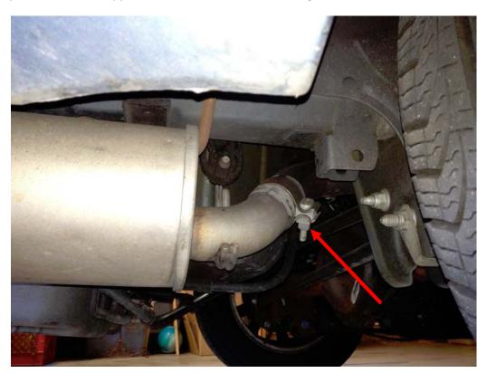
2. There are (3) hangers that support the muffler. Each hanger has (2) bolts securing them to the frame.
