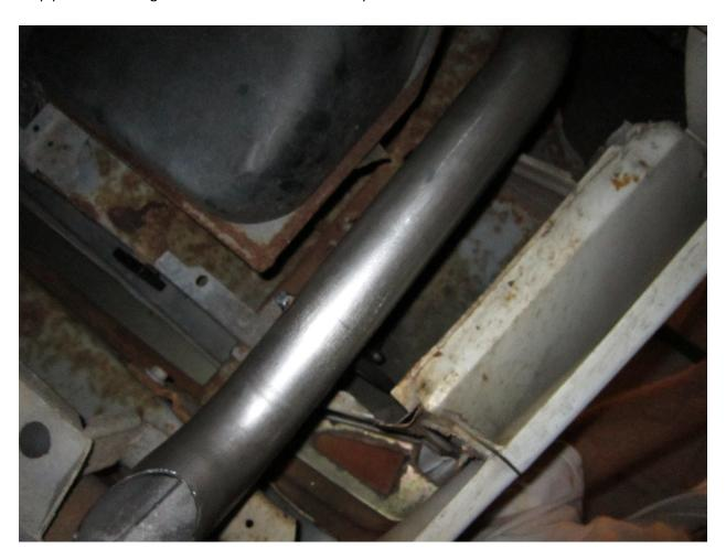
Step 9: Install the provided hangers (u-clamp) onto the tailpipe-muffler connection and tighten only when the tailpipes are in the correct position. Make sure all connections are secure and all hangers are attached properly.
