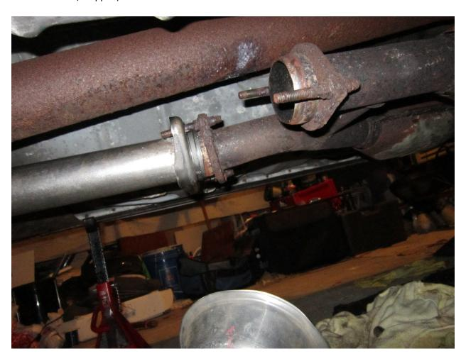
Step 6: Next reinstall the new muffler to the muffler hanger. Repeat for both sides.
