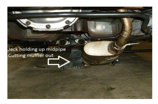
3. At this point you have two options undo the bolts holding the mid pipe to the catback or cutting the catback just behind the mufflers. After trial and error I found dropping the catback from the mid pipe made cutting easier. (
