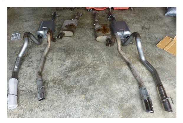
9. Apply anti seize to the threads on the clamps you are installing. Slide the clamps over the stubby exhaust ends at the back of the muffler cases.
