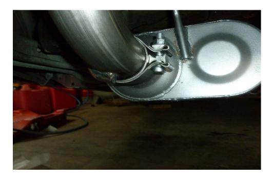
12. Attach the two studs through the flange where the mid pipe and muffler assembly meet. Leave these a little loose so that adjustments can be made.
