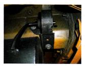
7) Install the OEM hanger bracket removed from the rear of the factory muffler onto the rear hanger of muffler #852467-229. Place the muffler up into position and connect the muffler inlet to the over-axle pipe. Bolt the hanger bracket to the frame using the OEM hardware. Connect the hanger on the front of the muffler to the factory mount on the vehicle.
