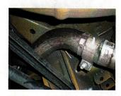
1) Loosen the 15mm nut on the clamped connection between the muffler and over-axle pipe and also the over-axle pipe to the factory Y-pipe.
