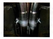
6) Place a 2½" clamp onto the slip-fit of over-axle pipe **#16679S** and slide onto the back of the right Scavenger outlet and support with a stand. Repeat this step with the left over-axle pipe **#16680S**.
