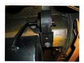
2) Unbolt the mounting brackets that mount the muffler to the frame (these are the two that connect the hangers on the *muffler body* to the frame). The mount connecting the hanger welded to the *inlet pipe* should remain bolted to the frame. Once these two hangers are unbolted, lower the muffler from the vehicle. Do not discard the OEM mounting brackets or hardware as they will be used in the installation of the new system. Lower the factory overaxle pipe from the vehicle and set aside.
