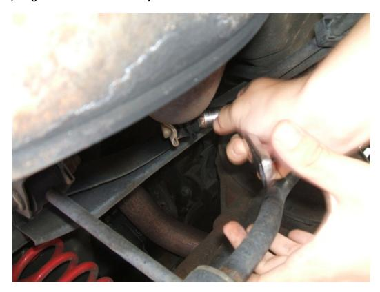
5. Now take the Pypes muffler delete system slide one of the supplied clamps over the end and attach it to the mid pipe on the car. Tighten the clamp enough to hold the exhaust on, but give it some play.
