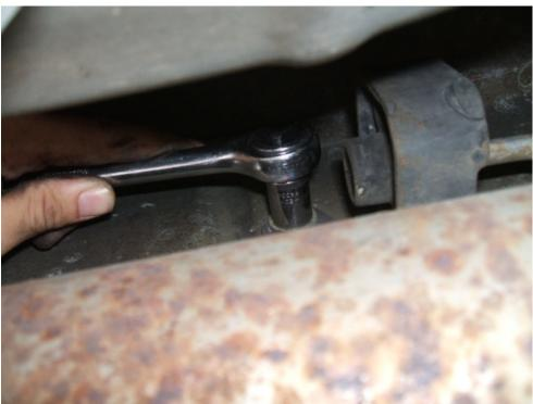
7. Make sure the mid pipe and muffler line up to your liking and are at the right height. Once you have verified that, you can tighten all the bolts and clamps. **Note: Make sure clamp is extremely tight. Tightening the clamp is where I needed the 15mm deep socket.**
