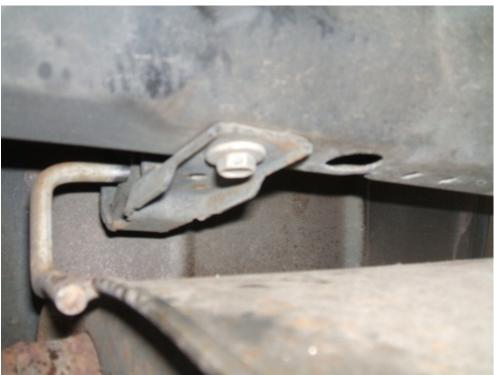
4. Once you have those hangers off use the 15mm socket to loosen the clamp holding the muffler to the mid pipe. Once you do that the muffler should slide off of the mid pipe. Note: I did not need the 15mm deep socket for this part, a regular 15mm socket worked just fine
