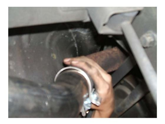
11. Now you can take the hangers and slide them over the exhaust hanger bars and attach them back to the frame rails. Again don't completely tighten make sure they are positioned to your liking and then tighten them down.
