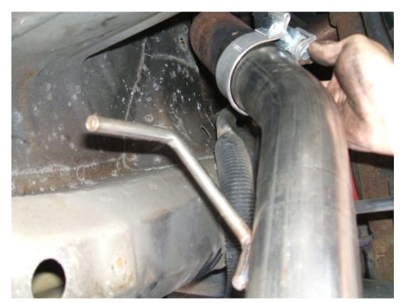
6. Now slide the hangers over the exhaust hanger bars and mount them back on to the frame rails. Again don't completely tighten them down.
