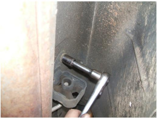
9. Once you have the hangers off loosen the clamp that connects the muffler to the mid pipe. Now it should slide right off.
