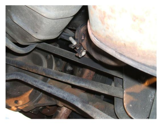
10. Take the Pypes muffler delete system slide a clamp on the end of the pipe and attach it to the end of the mid pipe. Tighten the clamp enough to hold it on the mid pipe but don't completely tighten it yet.
