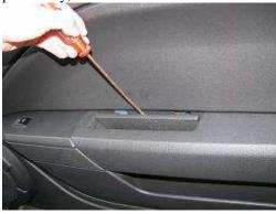
6. Remove the door lock bezel by slightly lift it up - a small screwdriver may be needed.
