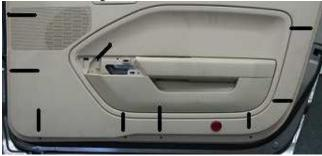
9. Lift up on the interior panel, removing it from the door. Remove any remaining electrical connections.
