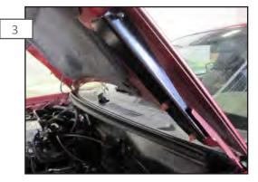
Slide the upper bracket between the rear-most nut and hood hinge and place it over the exposed front stud as shown.
