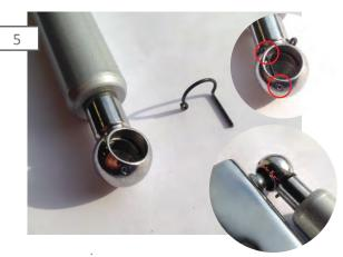
Remove the retaining clip. Place strut on the ball stud. Then reinstall the retaining clip.
