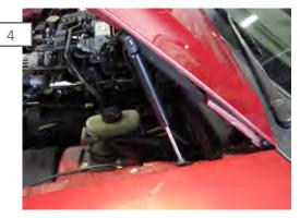
Pop the ends of the strut over the ball mounts on the brackets. Repeat steps 1-4 for drivers side. *(do not slam hood shut yet)* Check bumper/fender alignment by slowly lowering the hood. If okay, remove factory prop rod and enjoy.
