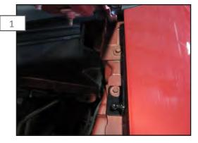
Prop your hood open and remove the 8mm fender bolt shown above (*Do not remove the rear-most bolt that secures the hood hinge*). Place the lower mounting bracket as shown and re-install the fender bolt.
