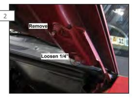
Use a 10mm socket to remove the forward most hood hinge nut. Loosen the rear nut about 1/4" (enough to slide in the upper mounting bracket).
