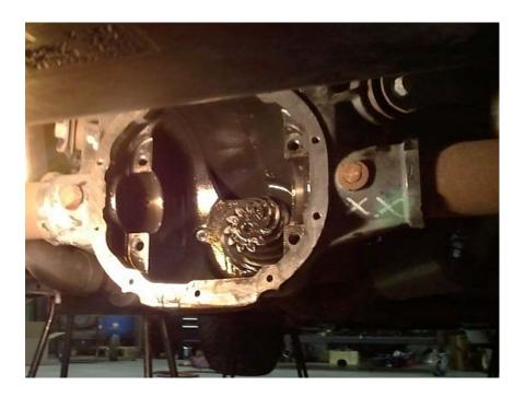
15. Before installing the new differential, we took some measurements from the bearing races on the driver side to the bearing races on the passenger side and then from the driver side to the ring gear.
