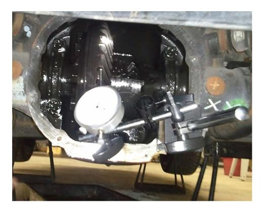
11. Next, you need to remove the (2) bearing caps on each side of your differential by taking off the (4) bolts using a 3/4" socket. Make sure to mark them so that you can put them back on the exact way they came off; otherwise they will not seat properly when you are reassembling the diff later.
