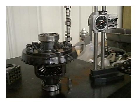
16. We measured 2.071 inches from driver side ring to race and then 7.708 in total width with the bearing races still on and took note of it (Picture shows our measurements for both OEM and the new diff; yours could vary.)
