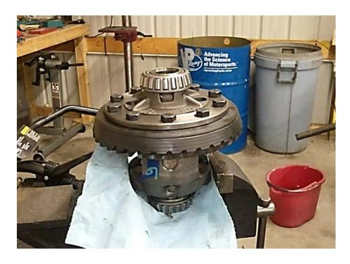
3. We then took our new measurements with everything installed on the differential. From driver side ring to race we measured 2.061 and the total width 7.722 inches. With these measurements, we were able to reuse the driver side shim, but we had to use other shims from our bearing kit because we had 10 thousandths of an inch less space on the passenger side. All of these measurements might vary depending on your car and year model.
