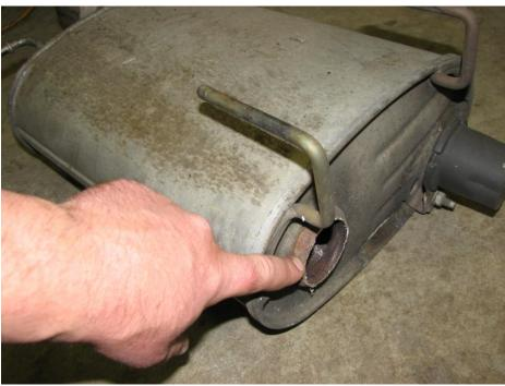
Figure 1: Cut off factory mufflers here
