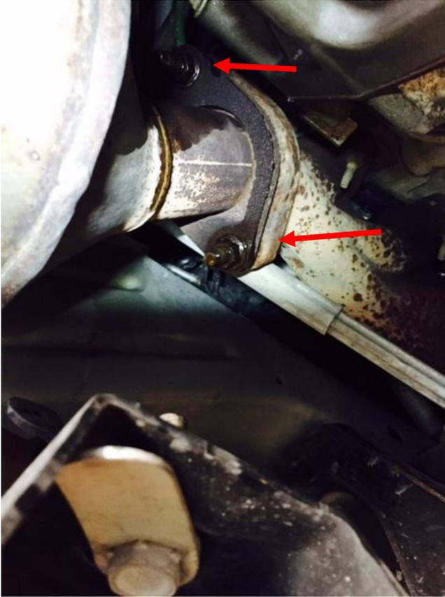
8. After you are done removing the 4 nuts (2 nuts on each side) slide your H-pipe off. It may be hard to get off so just wiggle it around until it slides off. Now it's time for the installation of your new X-pipe.
