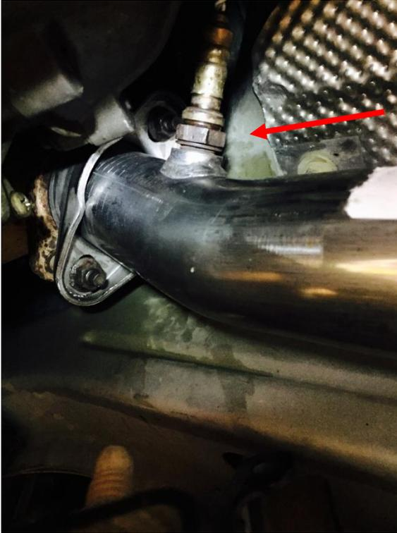
9. Now check for exhaust leaks. You can check for exhaust leaks by starting your car and putting your hand close by the connections of the rear pipes and the crossover pipe, the connections between the down pipes and the crossover pipe, and also the connections between the down pipes and the headers. If you feel any air coming out of those connections be sure to tighten the specific connection where you have a leak.
