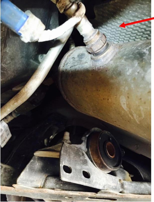
6. Next you're going to follow the stock H-pipe past the catalytic converter on both sides up to the flange mounts where the H-pipe is connected to the headers. There are 2 nuts on each side. You will need the 15mm Socket, swivel connection, and the Socket Wrench extensions to get past the catalytic converter.
