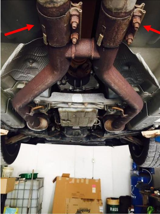
3. Loosen those 4 bolts on the sleeves with your 15mm socket and socket wrench but do not take the bolts off because you're going to want to slide them back on to your rear pipes so you are able to use them again to connect your new X-pipe.
