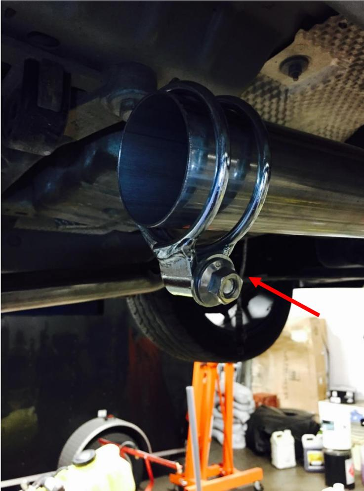
4. Now install your crossover pipe (the x-shaped pipe) to the down pipes. You may have to beat the inner portion of the crossover pipe with your hammer into shape to allow them to fit together.
