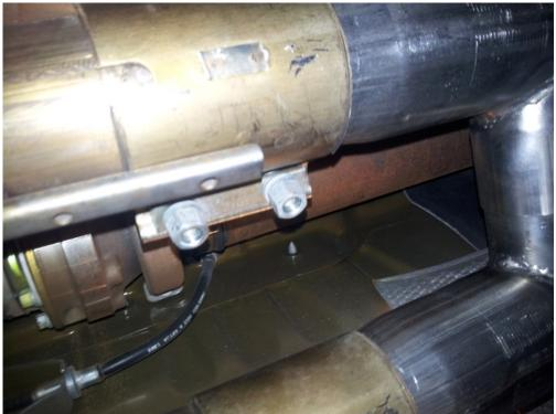
9. Install the U-bolt on the center section of the H-pipe. Make sure to orient the bolt so the ends face either the front or rear of the vehicle so there are no ground clearance issues. Using the ½" deep well socket start tightening the nut. Continue tightening until the outer pipe collapses onto the inner pipe forming a seal to exhaust gases. If desired some muffler putty can be used as well on the slip joint.
