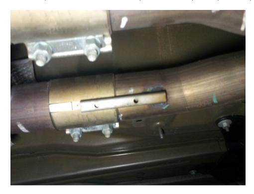
4. Locate the two clamps over the ball joints coming from the down pipes. Using a 13mm wrench break the two bolts free. This can be tricky because of the location but you should be able to achieve this with a little patience. After the two bolts are free use a pair of vice grips locked onto the bottom of the bolt that contains no threads and use the pliers to turn the bolts until the clamps are completely loose.
