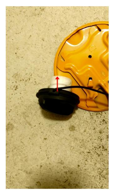
\*\*\*Leaving the gas cap off the new fuel door for now will make the installation easier\*\*\* 15. Unpack your new Fuel Door 16. Find this plate first
