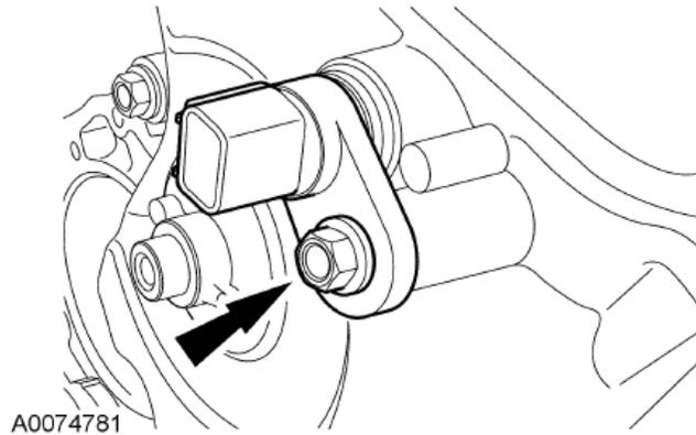
**STEP 11:** Connect the CMP electrical connector.
