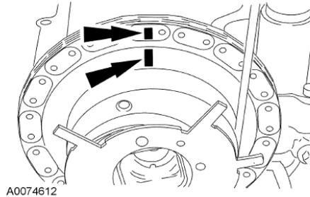
**STEP 4:** **NOTE:** Do not allow the camshaft roller followers to move out of position when installing the camshaft.
