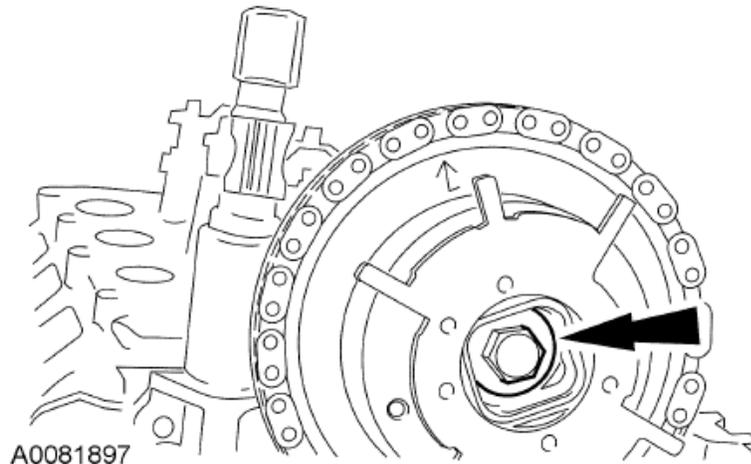
**STEP 3:**      **CAUTION:** Do not remove the timing chain wedge tool at any time during assembly. If the special tool is removed or out of placement, the engine front cover must be removed and the engine must be re-timed. For additional information, refer to Timing Drive Components in this section.
