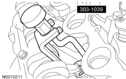
**STEP 9:**      **CAUTION:** The crankshaft cannot be moved past the 6 o'clock position once set or engine damage may occur.
