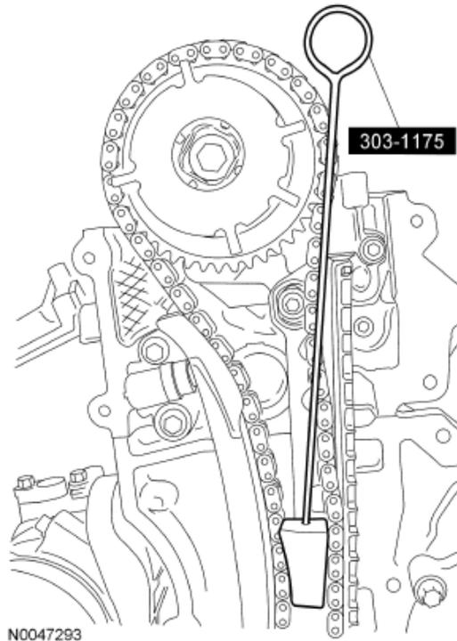
**STEP 7:**        Rotate the crankshaft a half turn counterclockwise and position the crankshaft damper spoke at the 12 o'clock position and the timing mark indentation at the 1 o'clock position.
