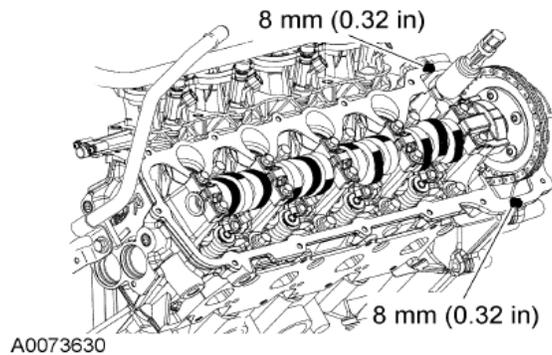
**STEP 2:**     Position the RH valve cover and new gasket on the cylinder head and tighten the bolts in the sequence shown below. Tighten the valve cover bolts to 10 Nm (89 lb-in).
