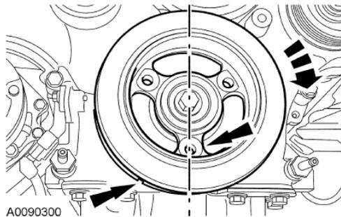
**STEP 10:**      **CAUTION: Engine is not freewheeling. Camshaft procedure must be followed exactly or damage to valves and pistons will result.**
