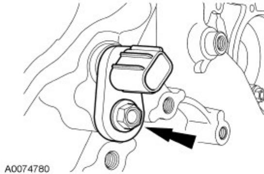
**STEP 11:** Connect the CMP electrical connector.
