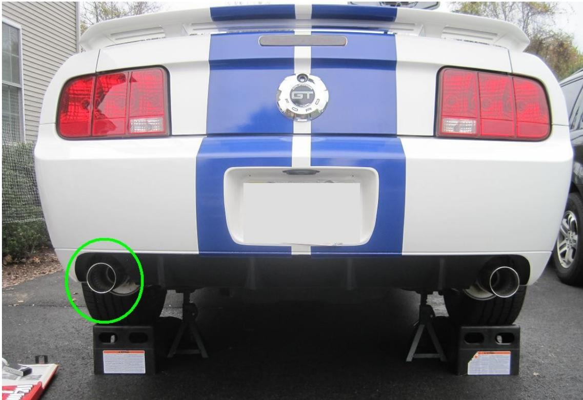
9. **Passenger side replacement:** The disassembly and assembly is almost the same as it was for the driver side, except there are only (4) bolts to remove: (2) toward the side of the muffler near the tail pipe and (2) bolts on the side of the muffler toward the front of the car. Follow the driver side instructions for removal and installation of the new passenger side FR500S axle-back:
