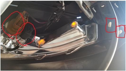
6. Remove the two (2) turn signal lamps by squeezing the white clips until the outer side pulls out, and then pull the tab out of the inner side. I put squares around the white clips in the picture directly above.
