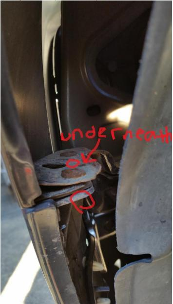
9. Using the 10mm socket, remove the two (2) upper bumper cover bolts from the vehicle. See picture directly below.
