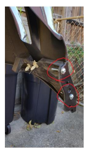
17. Installation of the new bumper cover is the opposite of the removal. Start by installing the two (2) 10mm bolts on the top of the bumper. Make sure that the large tabs on the bumper slide into the slot that is on the bottom of each headlight. I have circled one of the two (2) bumper tabs as it slides into the headlight slot in the picture directly below.
