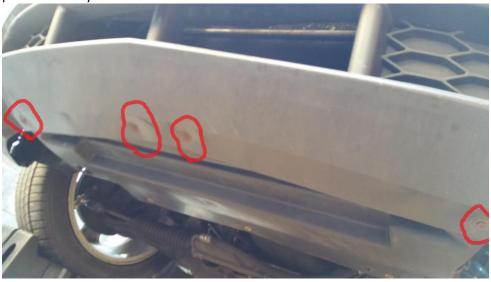
8. Using the 10mm socket and rachet, remove the two (2) front fascia to fender bolts from the each side of the vehicle. These are located at the connection between the fender and the bumper. Note: these
