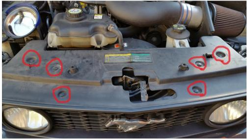
3. Remove three (3) screws at the bottom of each of the two (2) inner fender well covers with a Philipshead screwdriver. See picture directly below.
