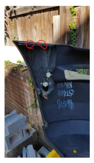
16. Install the old bumper reinforcement brackets that you just removed from the old bumper into the new bumper. I used stainless steel bolts, nuts and washers that I found in my garage. Make sure the head of the bolt is not too big since it needs to fit in between the bumper and fender (there is a cutout on the bottom of the fender for each). See picture directly below.
