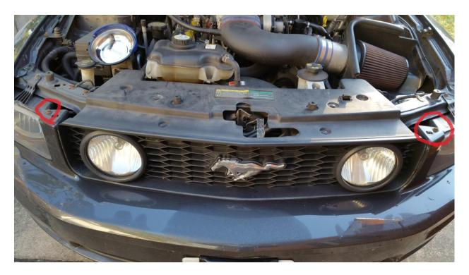
10. Pull the upper bumper cover mounts over the retaining tabs and pull the bumper cover partly away from the vehicle. The tabs are located directly next to the upper bumper cover bolts that you just removed.
