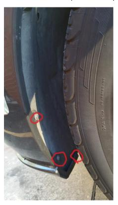
4. Remove the five (5) retaining clips from each of the two (2) <u>front</u> inner fender well covers. A flat-head screwdriver or panel remover tool will make this step easier. Remove each <u>front</u> inner fender well cover.
