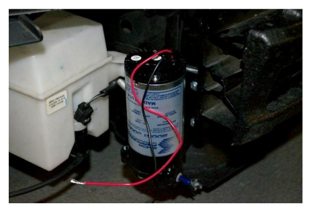
16. Take out the nylon tubing and test measure a length from the pump to the fitting that we sealed into the tank. Make a straight and square cut with your box cutter.
